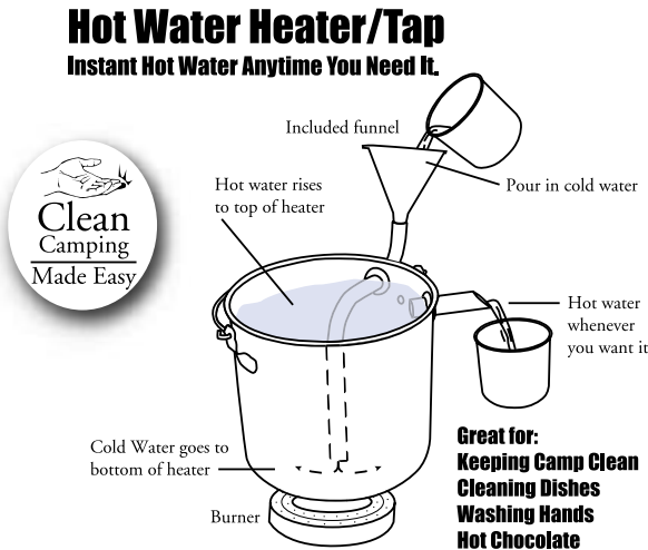
Figure 4-1 Hot Water Heater/Tap
